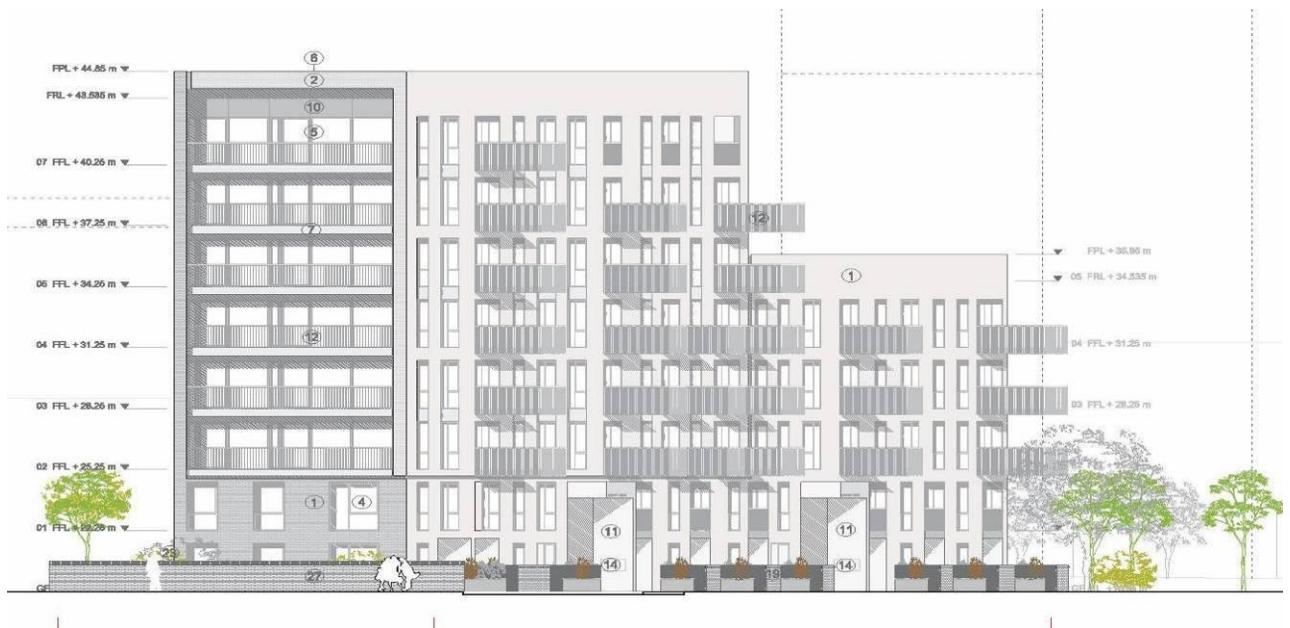
Figure 2: South facing elevation of Bridport House in Hackney showing eight-storey and five-story block of apartments
